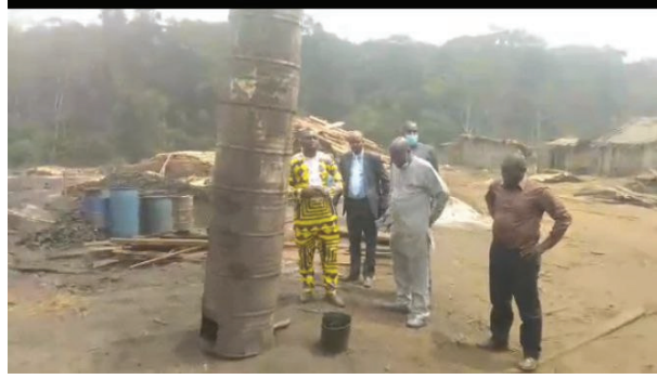
Casamance oven for charcoal, wood vinegar and biochar production
