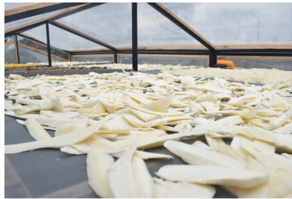
Figure 14 Internal view of a solar dryer complete with upper and lower shelves
