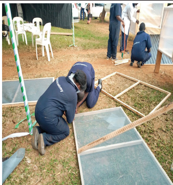
Figure 11 Making of trays for a solar dryer
