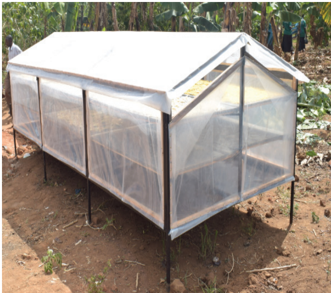
Figure 1 External view of a solar dryer:
