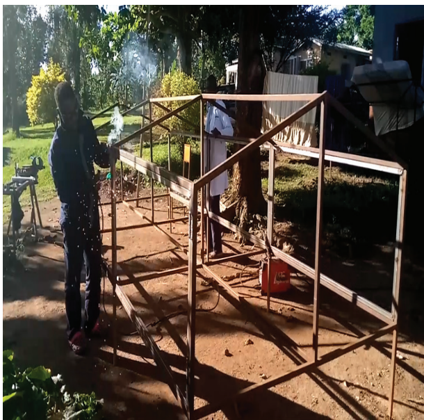
Figure 7 Youth Joining Frames of solar dryer
