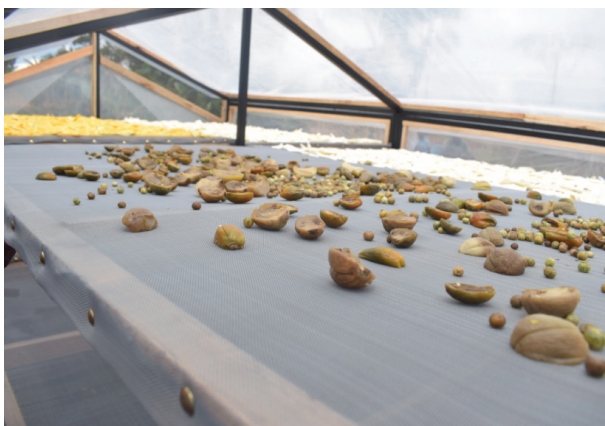
Figure 3 Interior view of a solar dryer: Showing trays having agriculture products
