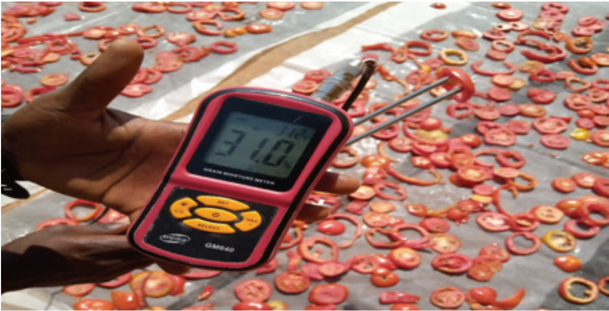
Figure 6a: sample digital moisture metre for use in monitoring drying rates
