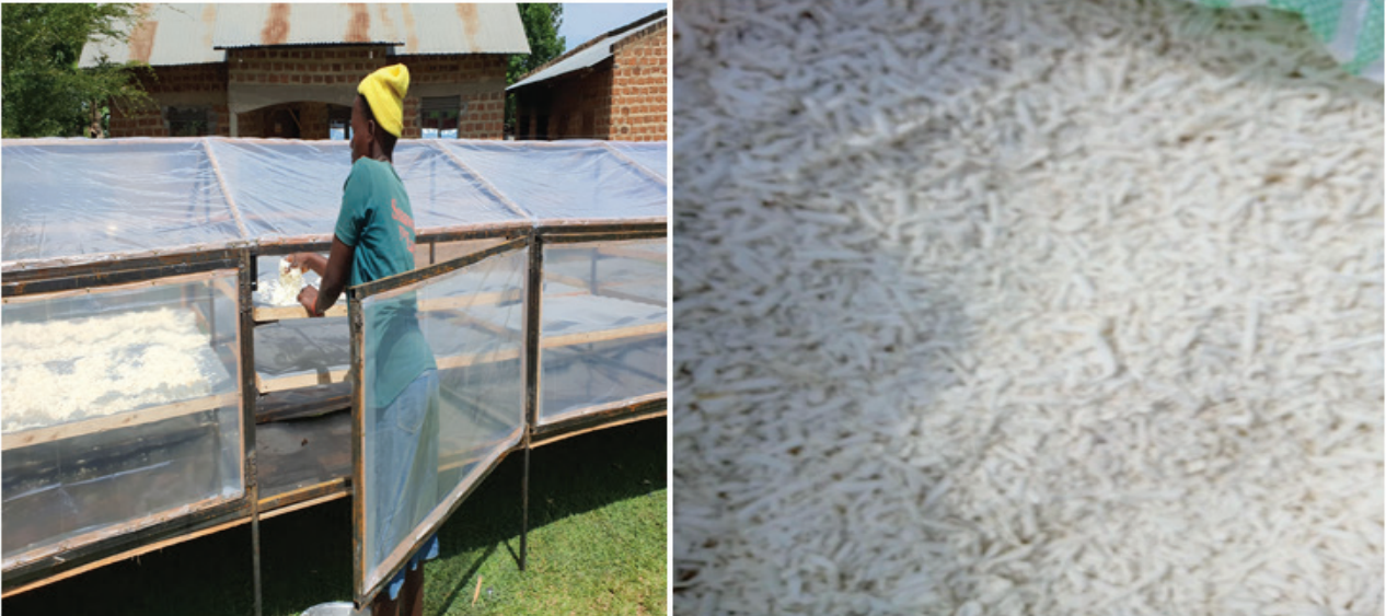
Figure 3a & 4a: cassava loading in process; loaded cassava spread over a tray to achieve uniform exposure.
