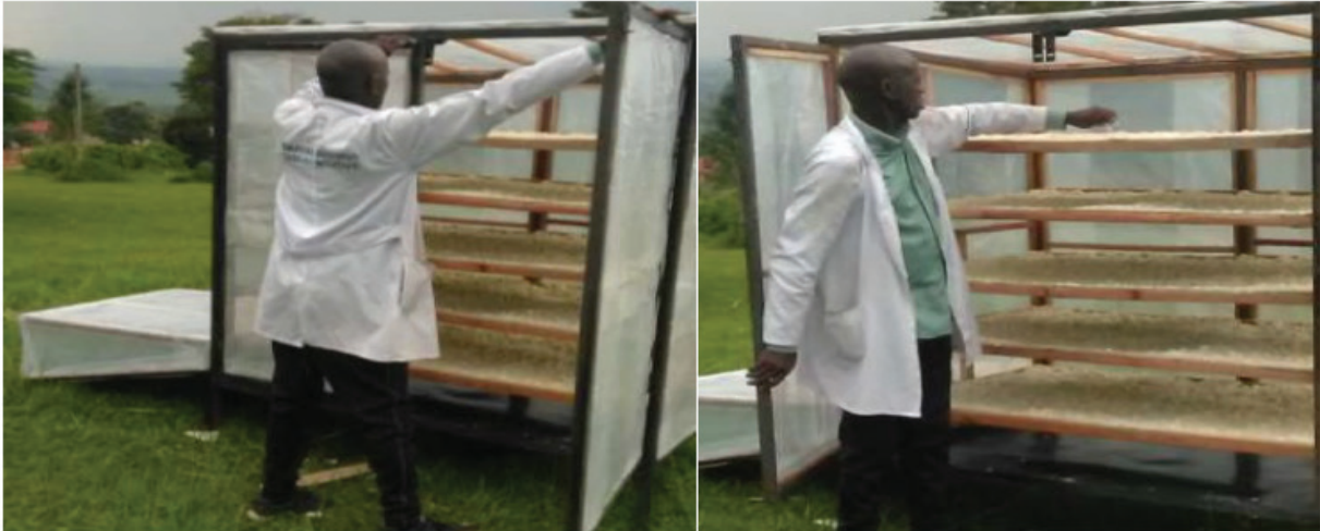
Figure 5a: fully loaded dryer demonstrating the spread of material to achieve uniform exposure
