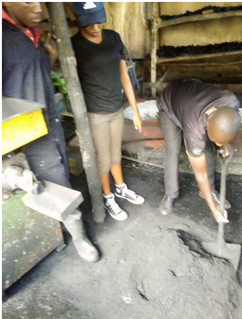
Mixing of the carbonized material
